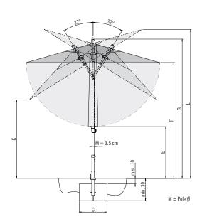
Loose cover max.  $10\,\text{cm},$  concrete thickness min.  $30\,\text{cm}$  (pay attention to frost depth), water outflow
